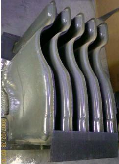
home. The by-products of combustion are water vapor,  $CO^2$ , and *carbon monoxide*. If there's a hole or crack in the heat exchanger, fumes are vented directly inside the home – usually with tragic results. There is NOTHING more important than determining the safety of your furnace each year through an **Infrared Camera Inspection** of your heat exchanger.
